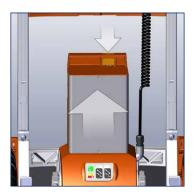
Press the release button and pull battery pack off.
