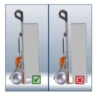
Make sure that the cargo is in tight contact with the C120.
