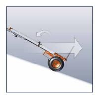
To slow down, tilt the C120 stronger so that the safety brakes can take effect.
