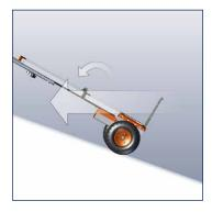
To slow down, tilt the C120 stronger so that the safety brakes can take effect.
