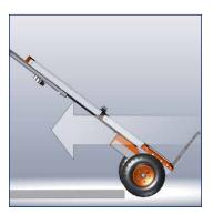
Overcoming obstacles. Approach the obstacle backwards with the C120 and then pull the C120 over the obstacle.
