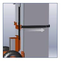
Secure the cargo on the C120 with the lashing strap 9.
