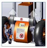
If the single-step mode (8) is active, the climbing leg is automatically stopped in neutral position (refer to section 5.8).
