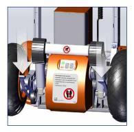
Deactivate the safety brake on both sides, respectively. To do so, push the brake lever downwards with the foot.
