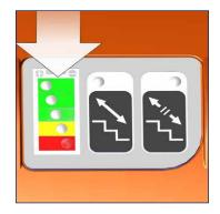
Red = battery depleted Charge battery. An acoustic warning sounds every 12 seconds. The capacity of the batteries will only last for max. 20 -30 steps!
