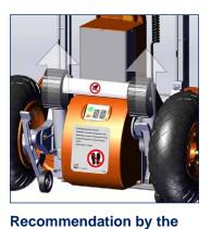
manufacturer: If the single-step mode is active, the climbing leg is automatically stopped in neutral position (refer to section 5.8).
