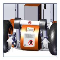
Activate the safety brake on both sides, respectively. To do so, push the brake lever upwards with the foot.
