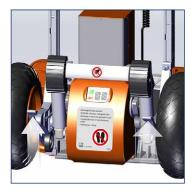
Activate the safety brake on both sides, respectively. To do so, push the brake lever 6 upwards with the foot.
