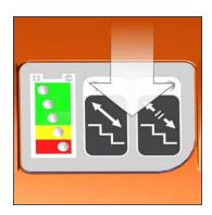
Depending on whether the continuous climbing mode or the single-step mode are active, the associated LED will be lit.
