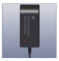
LED is lit red = battery is being charged.
