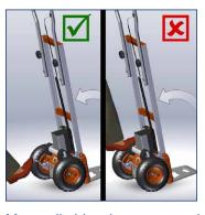
Move climbing leg to neutral position (refer to section 5.6) and tilt the C120 back.
